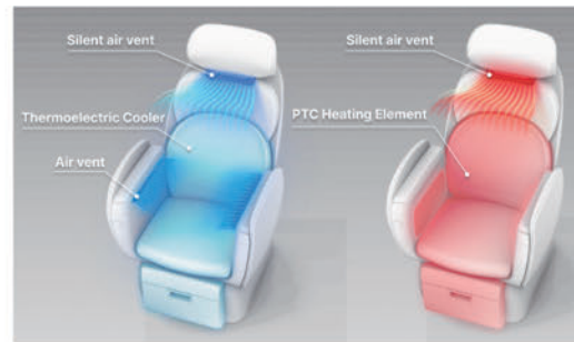
Fig. 3 The heating/cooling system of the seat concept
