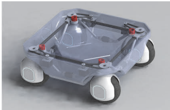
Fig. 14 Designed 4WIS system for proposing delivery robot
