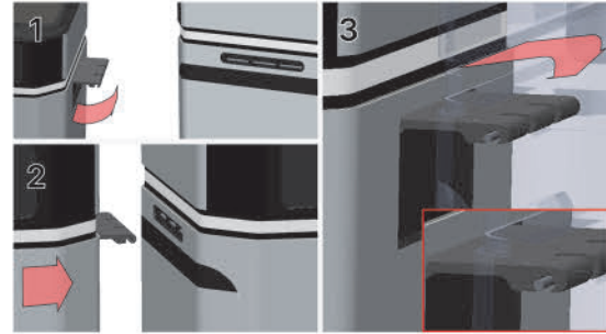
Fig. 22 Proposed lateral docking procedure
