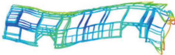
<2 nd Bending mode - 31 Hz>
