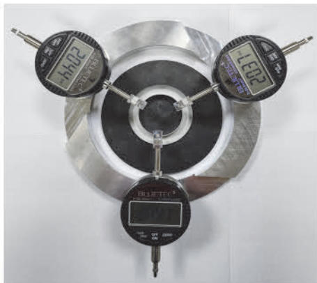
Fig. 7 Developed three-point contact-type inner diameter measuring device
