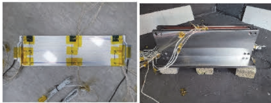
Photo. 1. Pouch type battery cell and ARC test setting
