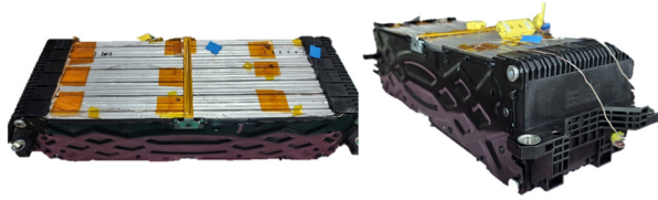
Fig. 5 Photograph of the battery module
