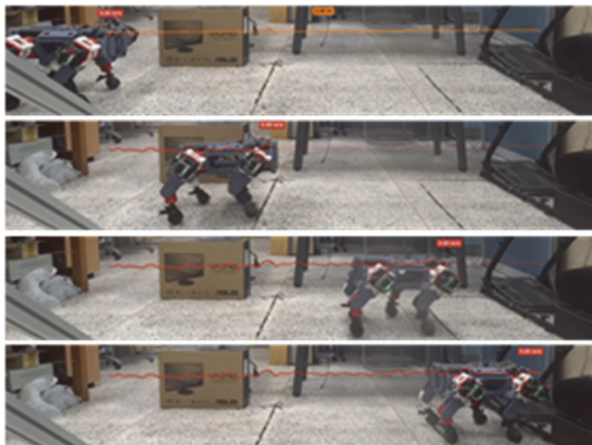
Fig. 12 Snapshots of trot gait during speed measurement
