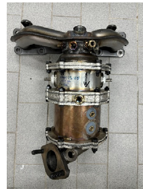
Fig. 3 EHC assembly before installation
