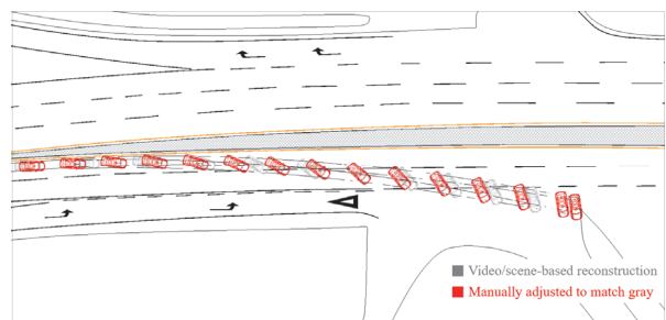
Fig. 10 Simulation based on tire marks and physical evidence, excluding EDR input (Case-2)
