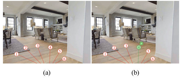
Fig. 7 Visual method for frontier selection. (a) Candidate waypoints are projected onto the egocentric view, (b) Candidate waypoints are directly evaluated and selected for the next waypoint
