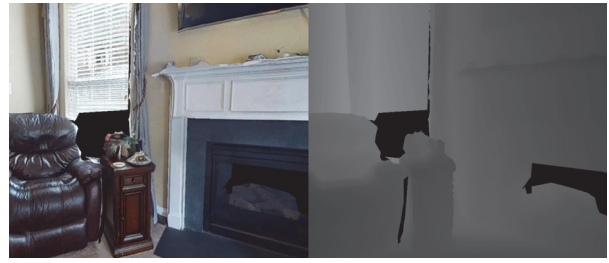
Fig. 9 An example of reconstruction artifacts (or defects) found in real-world scan datasets. The depth image (right) shows significant data loss also called ‘holes’ or ‘black cracks’
