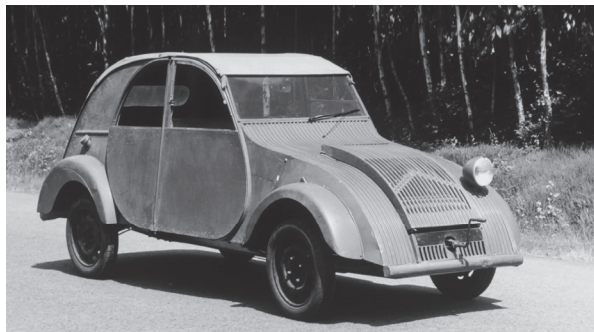
Fig. 13 Early prototype of Citroën TPV, 1938
