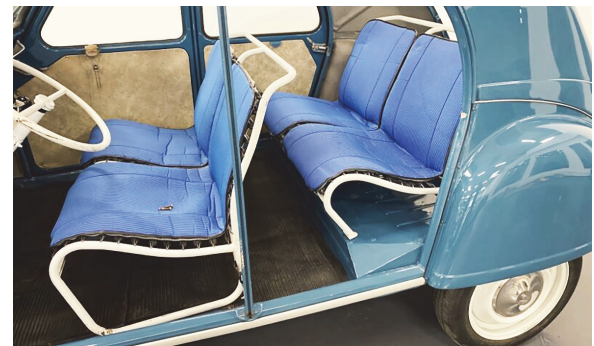
Fig. 19 Detachable doors and bench type seats of 2CV
