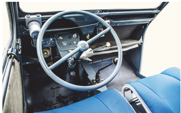
Fig. 18 Instrument panel of Citroën 2CV
