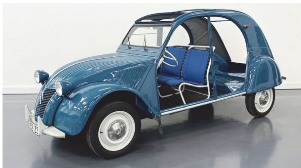
Fig. 16 Detachable side doors and flat floor of Citroën 2CV
