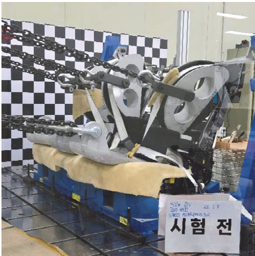
Fig. 1 Initial model prior to seatbelt anchorage strength evaluation
