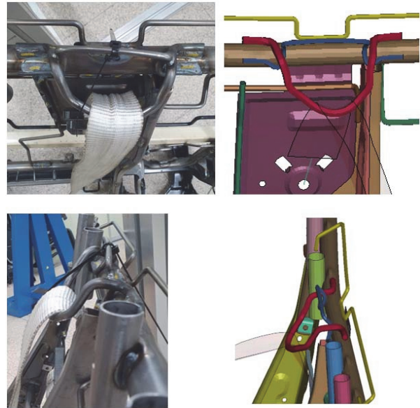
Fig. 14 Relative comparison between test results and FEA results under case #05 condition for the upper anchorage
