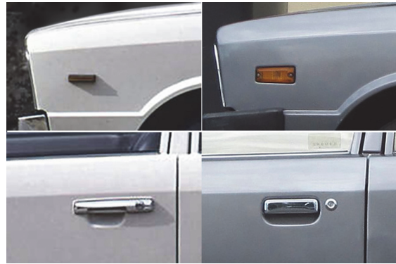
Fig. 9 Comparison details of turn signal lamps and door handles between 1976(L) and 1977(R) models
