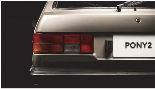
Fig. 21 Non-Euclidean curved surface of the upper part of semi notch deck of Pony 2 Hatch gate
