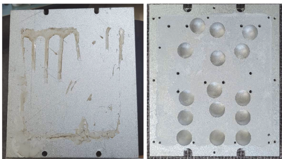
Fig. 1 Flat heat sink structure of motor controller (VEC500): (a) top surface, (b) bottom surface
