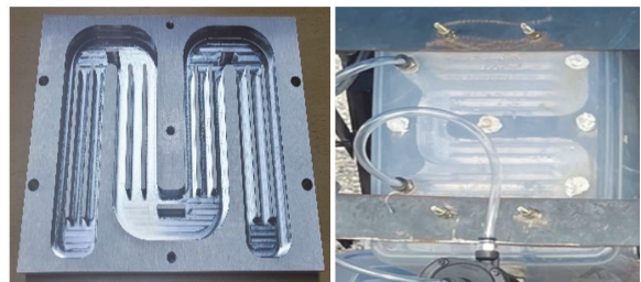
Fig. 2 Initial water cooling channel design and its installation on the vehicle
