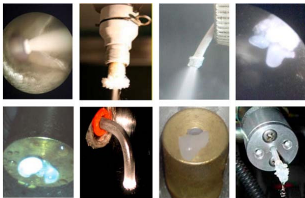
Fig. 1 Icing phenomena of liquid LPG injection
