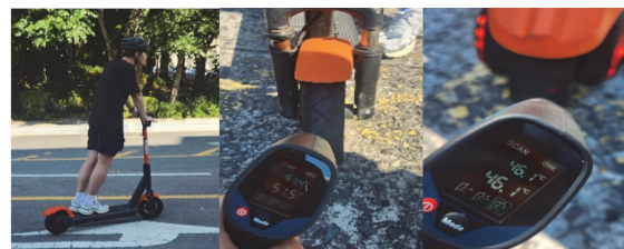
Fig. 4 Measurement of the surface temperature of a kick-scooter tire
