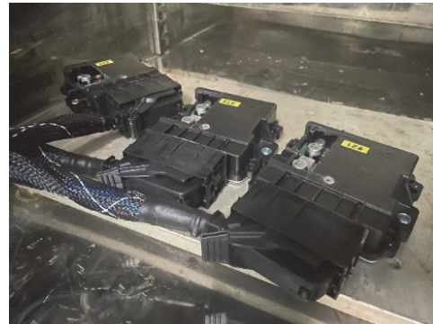
Fig. 5 Test sample for high-temperature operating life
