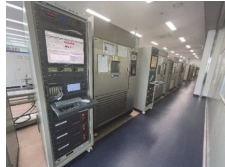
Fig. 4 Test equipment of high-temperature operating life
