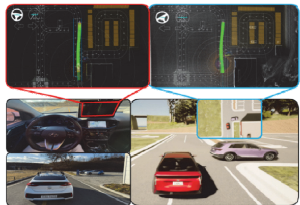
Fig. 16 Real-world and virtual environment validation experiments for autonomous driving systems
