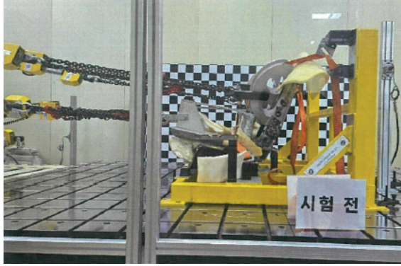
Fig. 1 Test model of seatbelt anchorage strength
