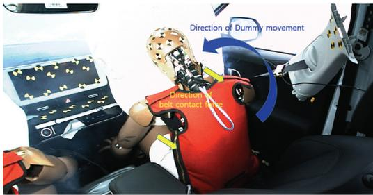
Photo. 4 Movement of the passenger dummy during 56 km/h MPDB test
