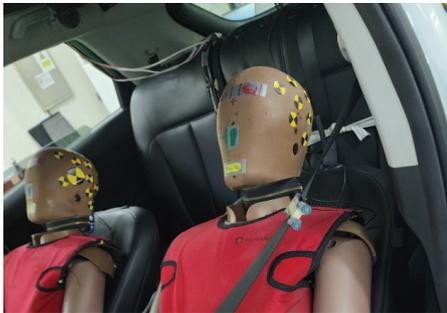
Remove the head restraint due to pushing the head by head restraint
