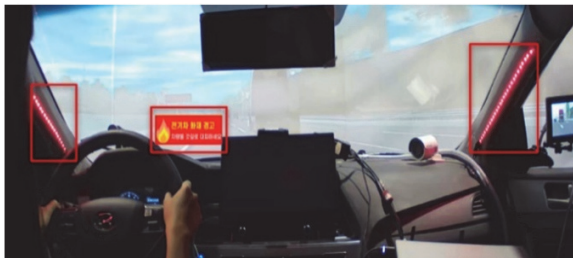
Photo. 2 Electric vehicle fire warning
