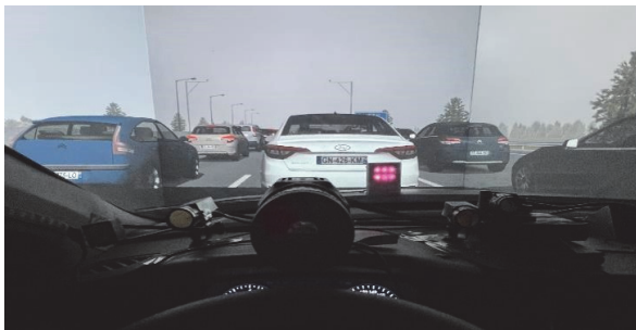
Fig. 3 Angry scenario(Traffic: heavy(LOS F), Average speed: 8-12 km/h, Weather: cloudy, Background sound: repeated horns)
