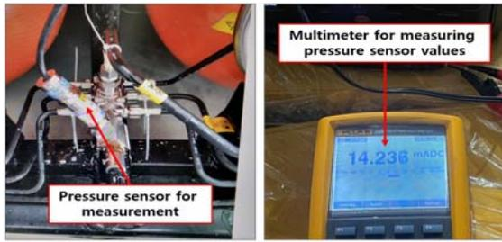
Fig. 1 Installation of pressure sensor for hydrogen tank pressure measurement
