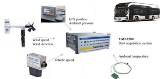
Fig. 4 RL(Road load) measuring equipment of fuel cell electric bus
