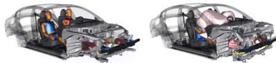
(c) Before crash of simulation (b) After crash of simulation
