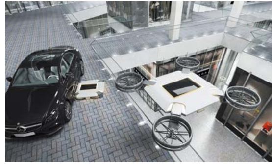
Fig. 26 The method of extending the rotors during flight and retracting them for charging
