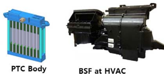
Fig. 12 PTC body and HVAC
