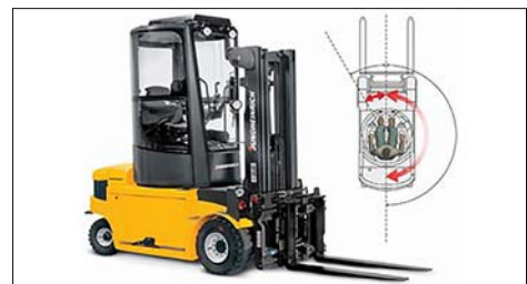
Fig. 13 Rear wheel steering type mechanism of a forklift
