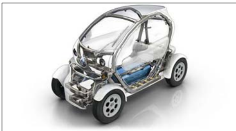
Fig. 10 Side frame structure from A-pillar to C-pillar
