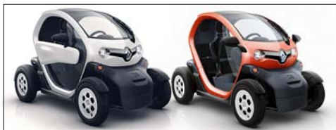
Fig. 11 Semi closed cabin structure of Twizy
