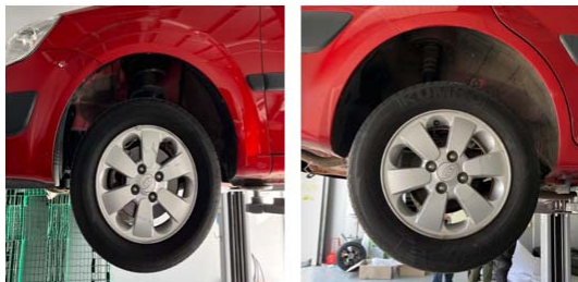
Fig. 2 Full-rebound condition of the front and rear suspension
