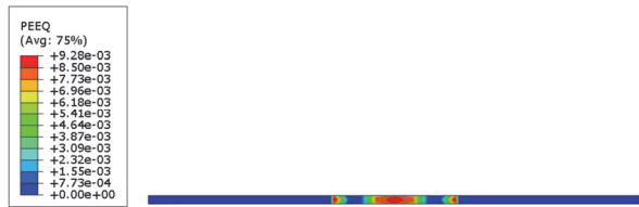
Fig. 17 Contour plot equivalent plastic strain for step 3 (bolt load 1,400 (N))
