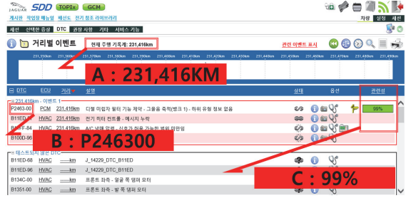
Fig. 5 Overview of OBD code
