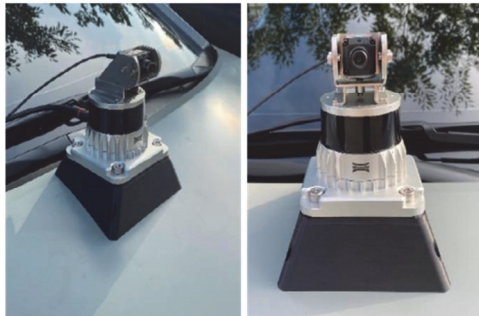
(b) LiDAR and camera sensor mounting
