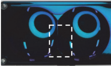
Fig. 17 Improved LiDAR after high temperature and humidity test sample
