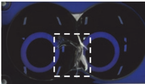
Fig. 13 High temperature and humidity test sample
