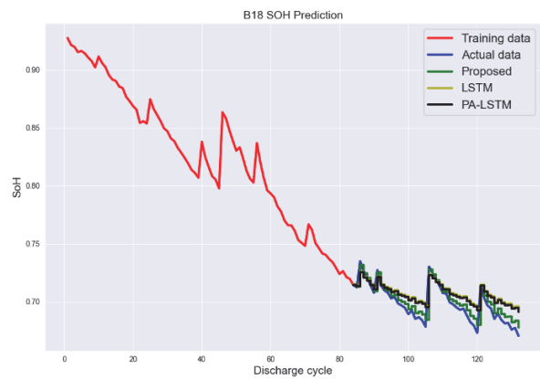
Fig. 6 Comparison of SoH estimation results among the proposed model, LSTM, 12) and PA-LSTM 13) with NASA battery cell B18
