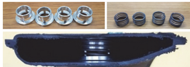
Photo 3 Cross-sectional photograph of the variable resonator
