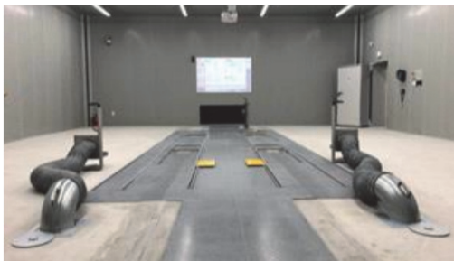
Photo 2 Noise test by chassis dynamometer
