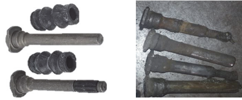
Fig. 10 New parts and damaged parts of guide pin
