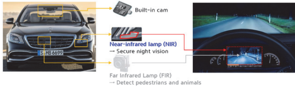
Fig. 2 Basic configuration of the night vision system
