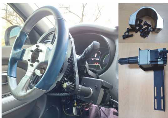
Fig. 4 Step motor and timing pulley to control the steering wheel
