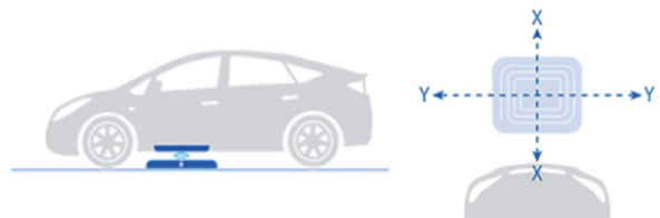
Fig. 1 WiTricity 17) wireless charging platform
