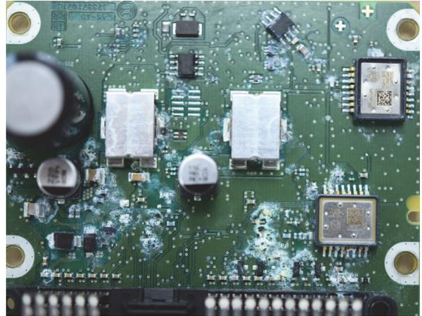
Fig. 4 Corroded states of RCM's circuit board
