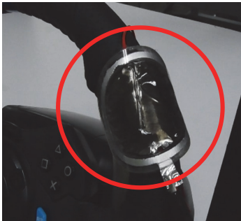
Fig. 4 Prototype of steering wheel vibration generator
