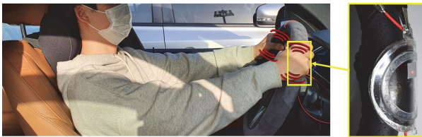
Fig. 11 Demonstration picture of the proposed steering wheel vibration generator
