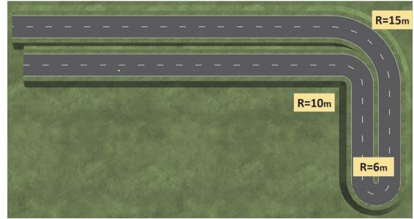
Fig. 9 High curvature test scenario
