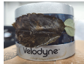
Fig. 18 LiDAR surface is contaminated with leaves
