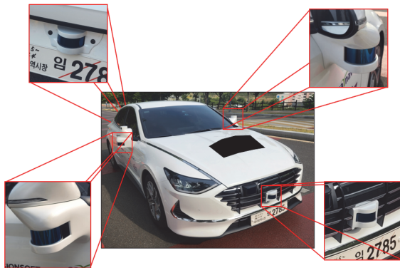
Fig. 5 LiDAR attached to autonomous vehicle in various ways
