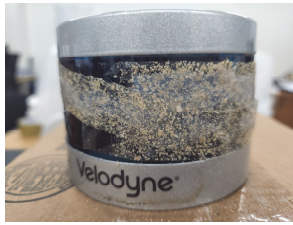
Fig. 15 LiDAR surface is contaminated with soil
