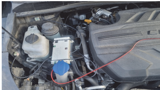
Fig. 13 Installation of IoT edge in engine room ( https://youtu.be/Qlj7xWE5ZSc )
