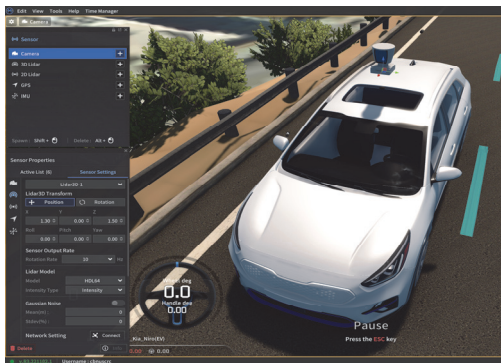
Fig. 13 Lidar sensor attachment installed in actual vehicle design position
