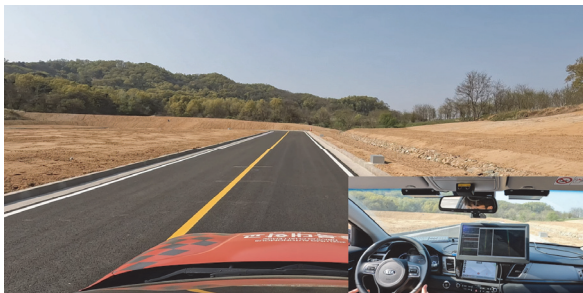
Fig. 10 Test evaluation with longitudinal and lateral control inputs for verification of driving in correct way and lane keeping
