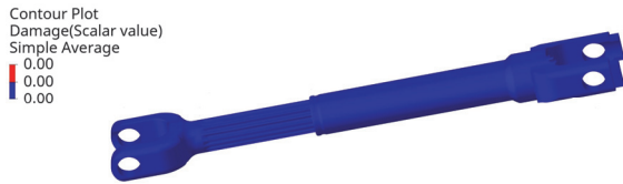
Fig. 22 Damage plot of intermediate shaft assembly as results of torsional durability analysis
