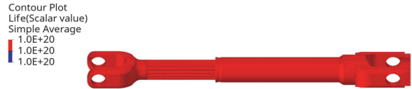
Fig. 19 Life plot of intermediate shaft assembly as results of rotational durability analysis
