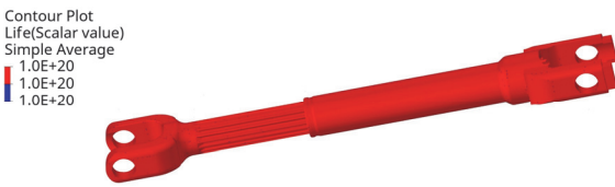
Fig. 23 Life plot of intermediate shaft assembly as results of torsional durability analysis
