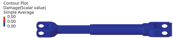
Fig. 18 Damage plot of intermediate shaft assembly as results of rotational durability analysis
