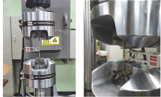
Fig. 3 MTS 810 material test system
