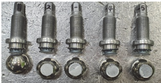
Fig. 7 Ball stud bending test samples
