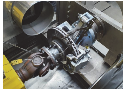
Fig. 11 Test configuration of brake dynamometer
