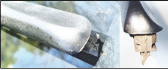
Fig. 9 Deformed rubber strip causing chattering
