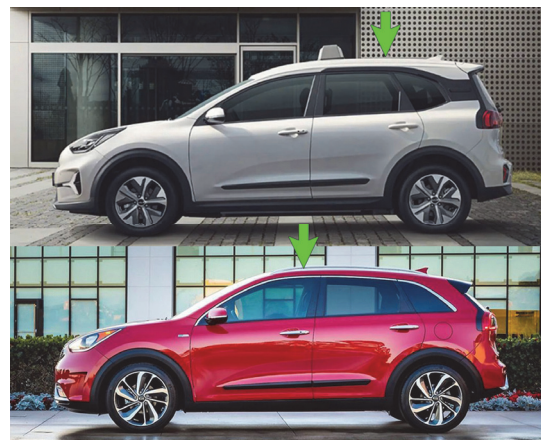
Fig. 10 Roof slope peak position and height difference between Kia Niro Plus PBV(above) and old Niro(below)
