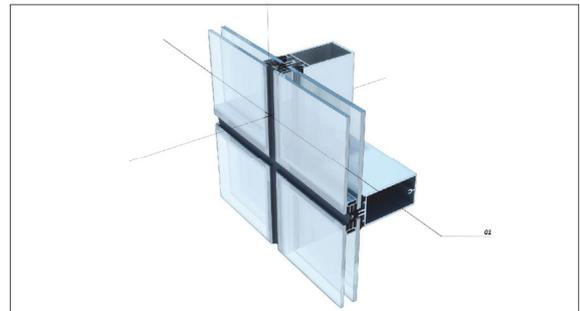
Fig. 9 Pair glasses and wall assembly of curtain wall structure
